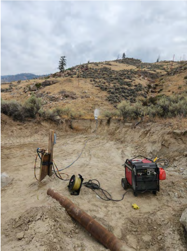
7. Pumping test on WTN 124408. Discharge hose ran to the east to discharge at top of bank into unnamed draw along north of site. View looking northeast.
