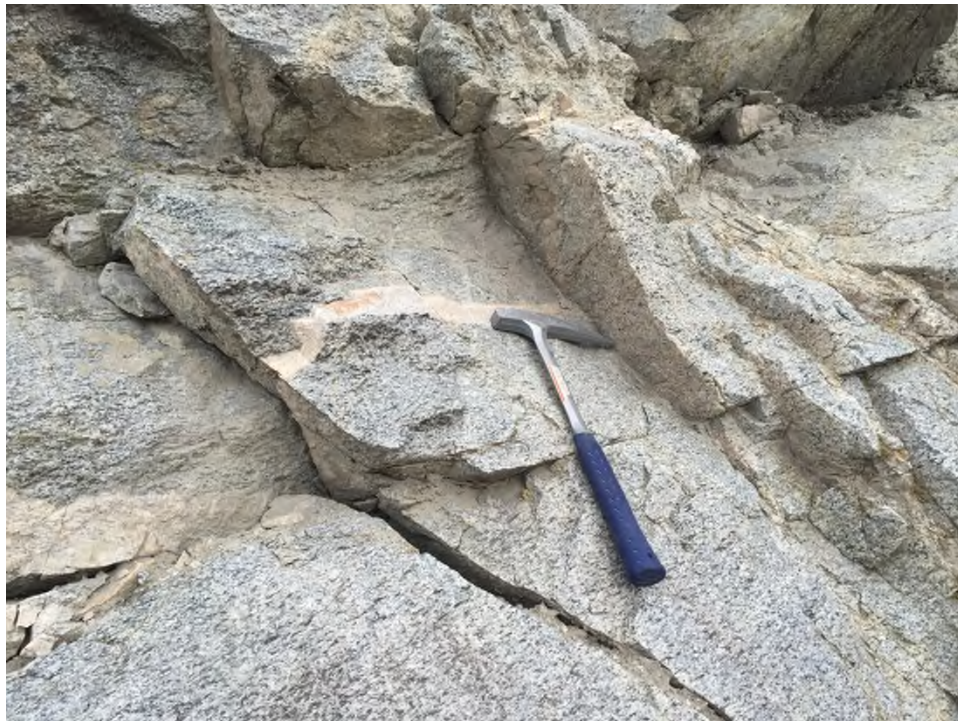
Photo 2 Discontinuity mapping of rock outcrops during mapping.
