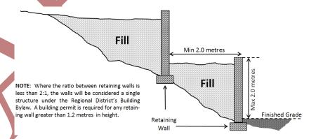
Figure 3 - Retaining Wall Illustration
