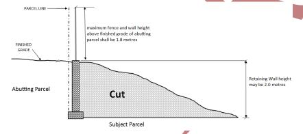
Figure 7.29.5: Retaining Wall in a Setback Illustration
