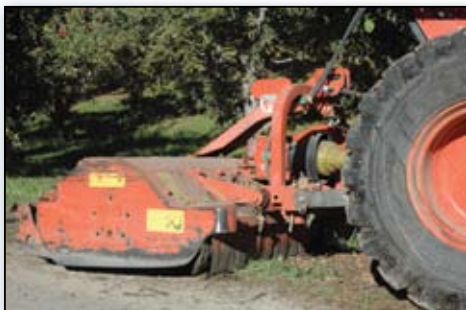
A FLAIL MOWER can be used by growers as a tractor attachment to create mulch from vineyard, orchard and berry crop prunings or from ground crops.
