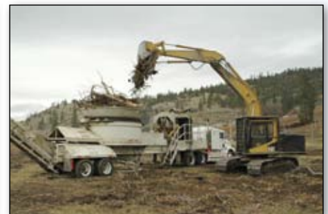
A TUB GRINDER is the largest of the equipment used to grind, chop and shred wood waste. There may be one at your local landfill. If required, contact local government to see if it is available to come your site.
