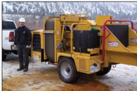
A PORTABLE CHIPPER can be rented or you can employ a local contractor. chippers vary in size. Some chippers can chip wood waste up to 15" in diameter. Chip size produced depends on the screen, but should be between 1"-2".
