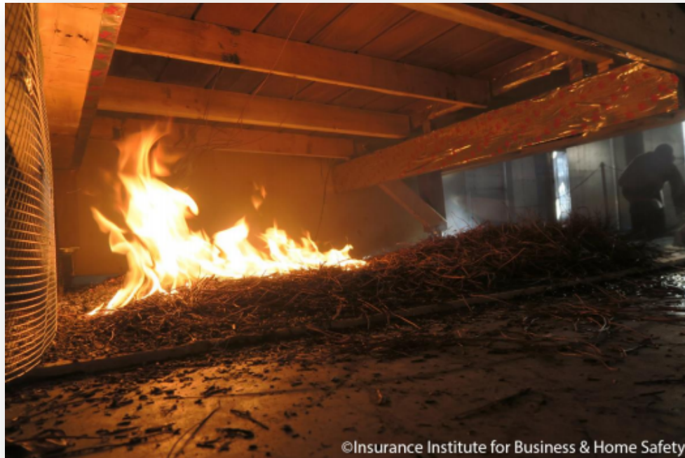
Figure 25 This photo was taken during testing by the Insurance Institute for Business & Home Safety. A full-scale home model placed in a burn chamber was subjected to an ember blizzard to test the effect of embers and ember accumulation on structures during a wildfire. Deck boards permitted embers to pass through the between-deck-board-gaps and ignited combustible accumulations under the deck. A deck or porch where the underside is completely open offers no resistance to ember accumulation. [Photo: (Quarles & Standohar-Alfano, 2017)]
