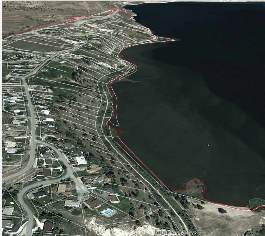
Figure 30 Three-dimensional Google Earth image of the area approximated in Figure 29. Significant portions of property lie downslope above the KVR trail where slopes are up to 70%. Fuel management on these slopes would be challenging.
