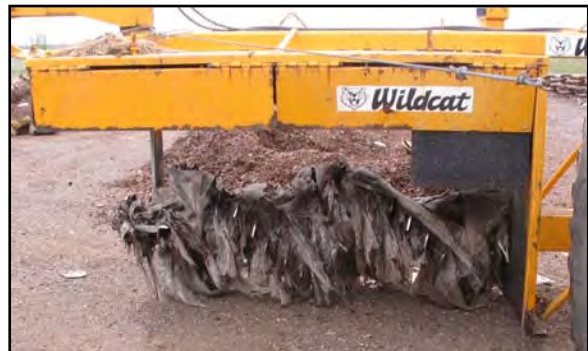
Exhibit 5- 7: Plastic wrapped around the flails on a windrow turner.
