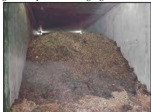
Exhibit 6- 9: Aerated static pile composting being done inside an enclosed concrete "tunnel".
