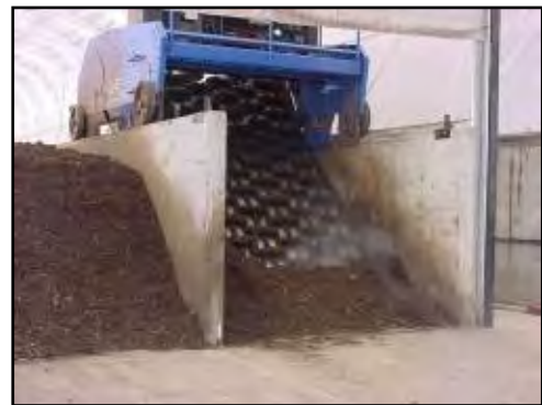
Exhibit 6- 10: Channel composting system used to process animal manures.
