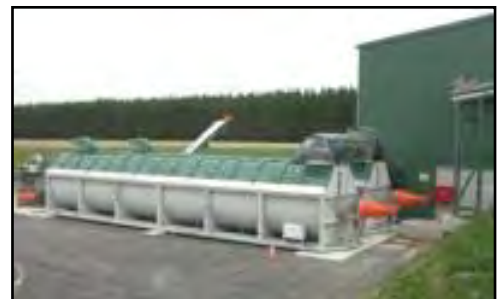
Exhibit 6- 14: Hot Rot's mid-sized composting unit.
