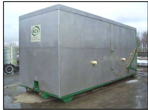
Exhibit 6- 11: Containerized composting system manufactured by Engineered Compost Systems.
