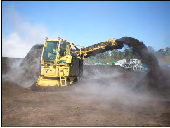
Exhibit 6- 8: A self-propelled Vermeer windrow turner equipped with a horizontal cross conveyor.
